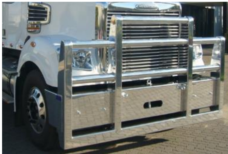
Figure 9: Truck fitted with FUPs bar
