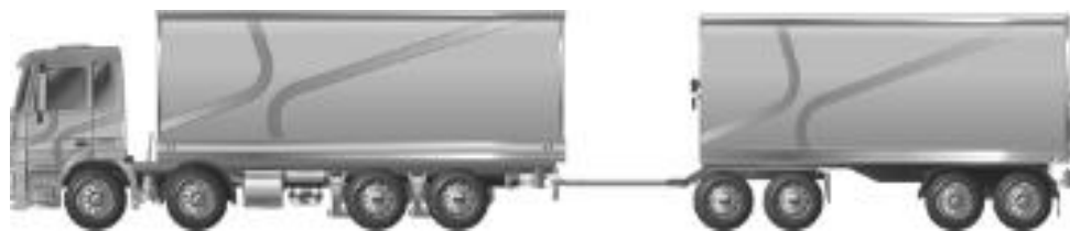
Figure 39: Example twin steer truck (Code 73 – 4 Axle Twin Steer Rigid Truck & 4 Axle Dog Trailer)
