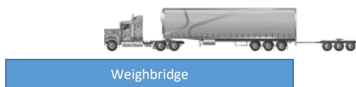
Figure 11: Semitrailer and dolly weighed with dolly off the weighbridge
