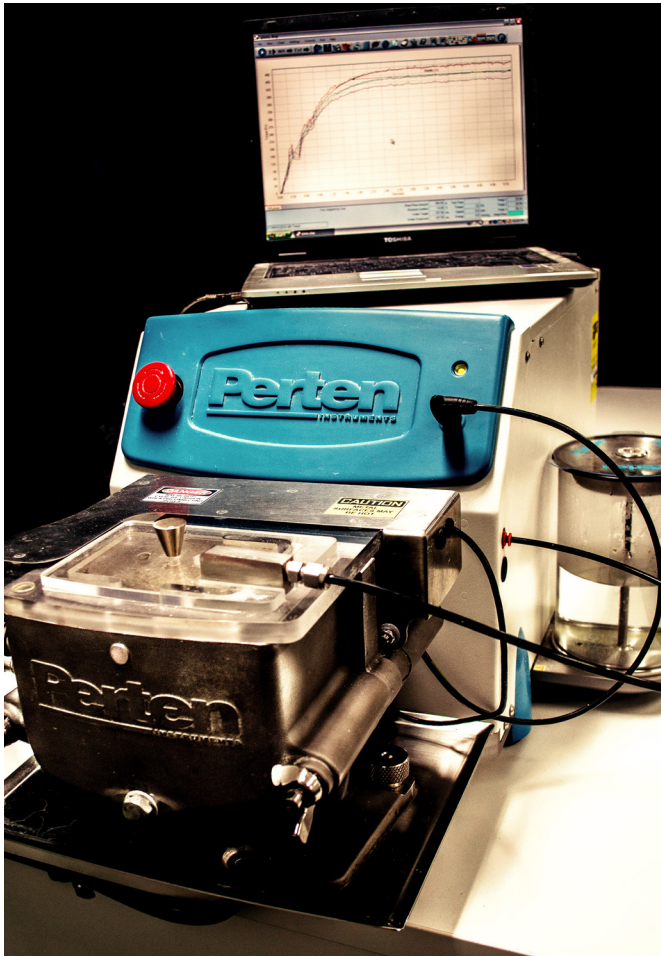
Perten Dough Lab conducting a farinogram.
